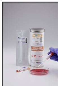
The Microbiologics® KWIK-STIK™ features a lyophilized microorganism pellet, reservoir of hydrating fluid and inoculating swab
