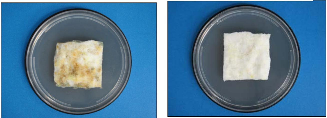
**Pictured above:** Untreated (left) and treated (right) foams tested in the **ASTM G-21** using a mixed suspension of *Aspergillus niger*; *Aureobasidium pullulans*; *Chaetomium globosum*; *Penicillium funiculosum*; *Trichoderma virens*
